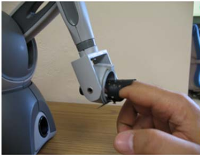
Figure 1. Omni® Haptic Interface (SensAble Technologies, Inc.) Modified for the Haptic Modules with a Finger Gimbal
